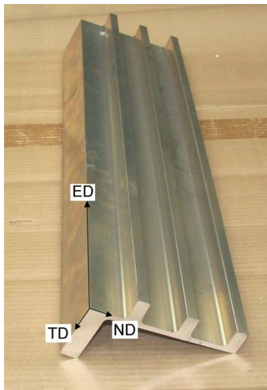
Fig. 1 Photo of Mg extrusion and orientation designation (samples were taken from the thick section)
